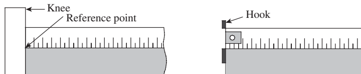
Fig 4.9 Correct ways of using a rule with attachments
