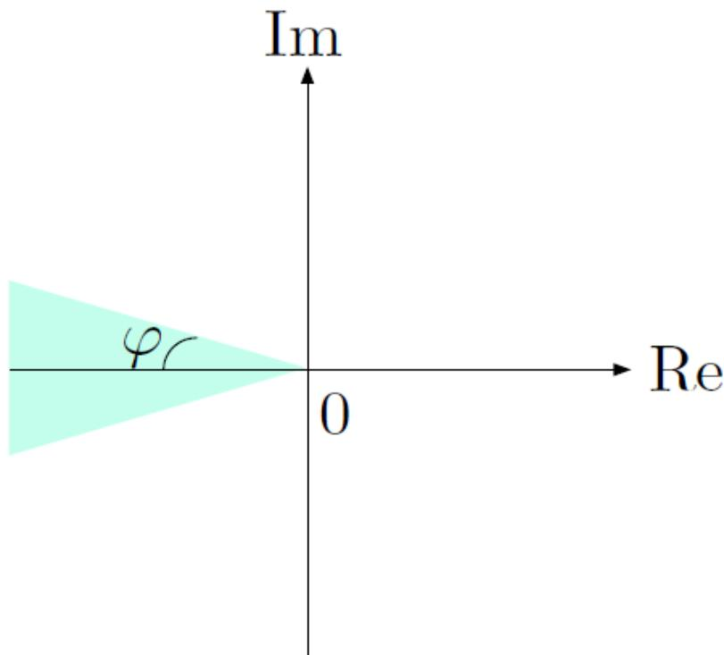
$$\begin{aligned}\frac{\zeta}{\sqrt{1-\zeta^2}} &= \frac{\omega_n \zeta}{\omega_n \sqrt{1-\zeta^2}} \\ &= \frac{\sigma}{\omega_d} = \cot \varphi\end{aligned}$$
