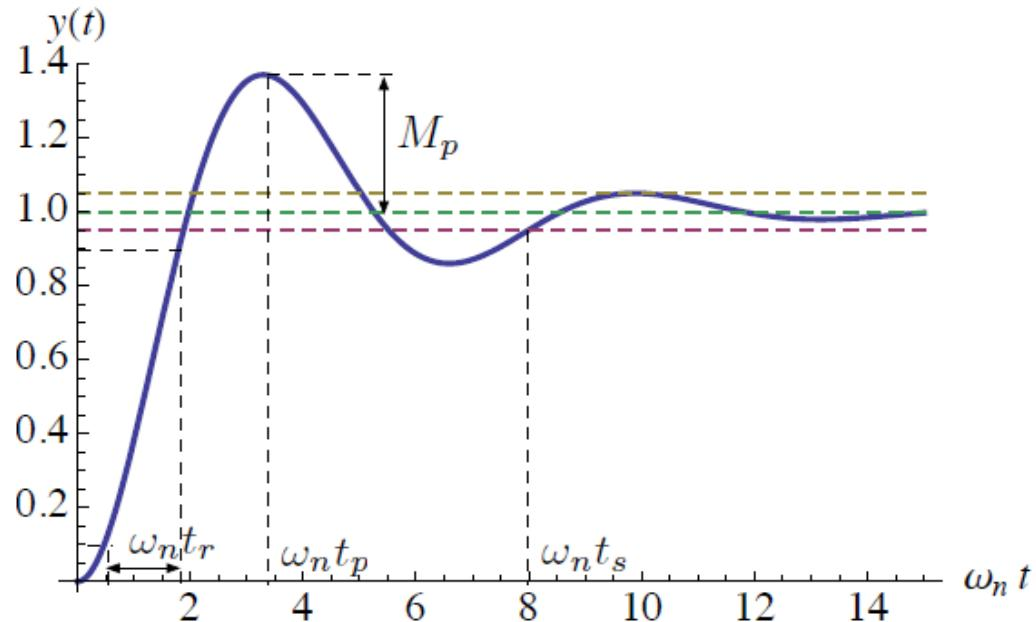
$$t_s = \min \left\{ t > 0 : \frac{|y(t') - y(\infty)|}{y(\infty)} \leq 0.05 \text{ for all } t' \geq t \right\} \text{ (here, } y(\infty) = 1\text{)}$$
