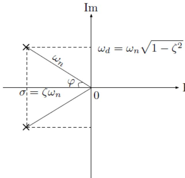
$$\begin{aligned}\omega_n^2 &= \sigma^2 + \omega_d^2 \\ \zeta &= \cos \varphi\end{aligned}$$
