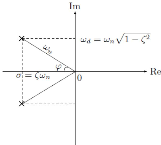
Step response:  $y(t) = 1 - e^{-\sigma t} \left( \cos(\omega_d t) + \frac{\sigma}{\omega_d} \sin(\omega_d t) \right)$
