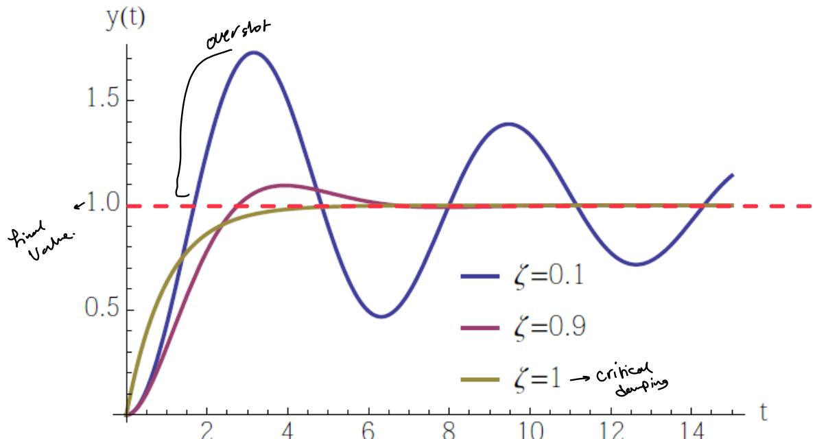
The parameter  $\zeta$  is called the *damping ratio*
