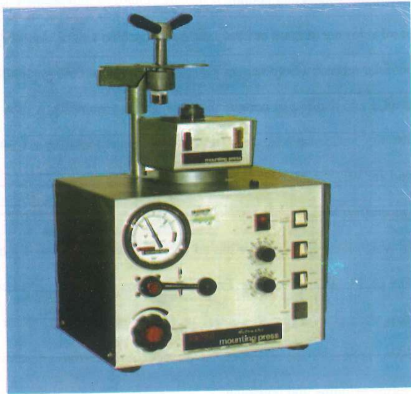
Figure 4. Automatic Mounting Press for Hot Mounting Purposes.
