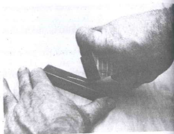
Figure 6b. The sample is now scratched against the mild steel as a further test and it does scratch the mild steel
