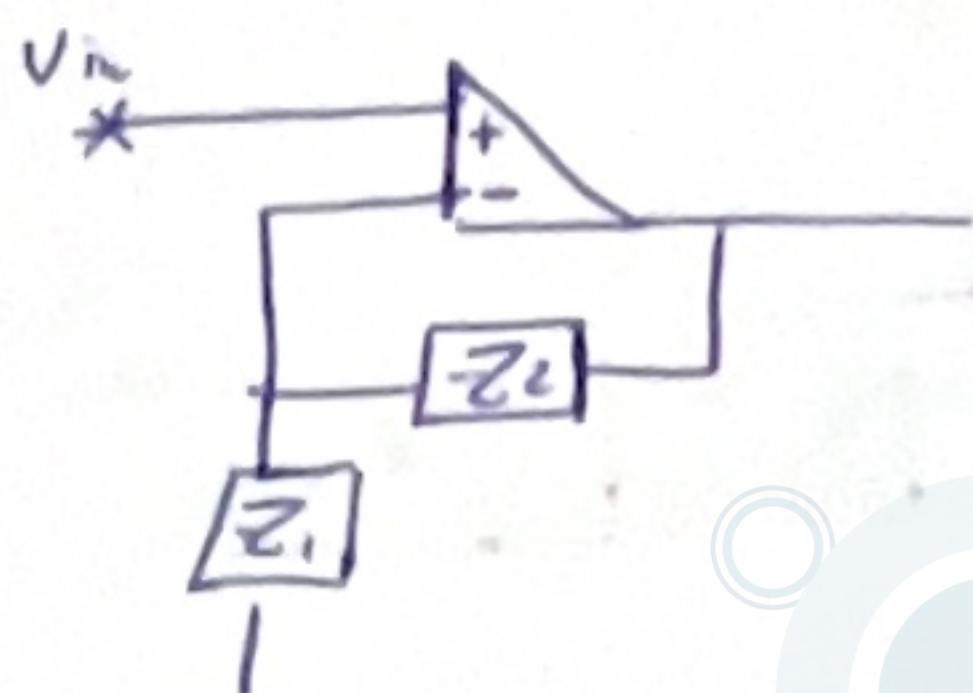
$$\text{Inverting } TF = \frac{V_{\text{output}}}{V_{\text{input}}} = -\frac{Z_2}{Z_1}$$
