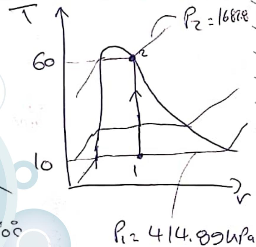
**Q.2 (10 points)** A piston-cylinder arrangement contains water at  $100^{\circ}\text{C}$  and 85% quality with a total volume of 1 lit. Heat is added until the piston touches a linear spring at the instant the volume is 1.5 lit. Heating continues until the pressure reached 200 kPa. If the piston diameter is 150 mm and the spring constant is 100 kN/mm, calculate the total work done and total heat transfer. Sketch the P-V or T-v.
