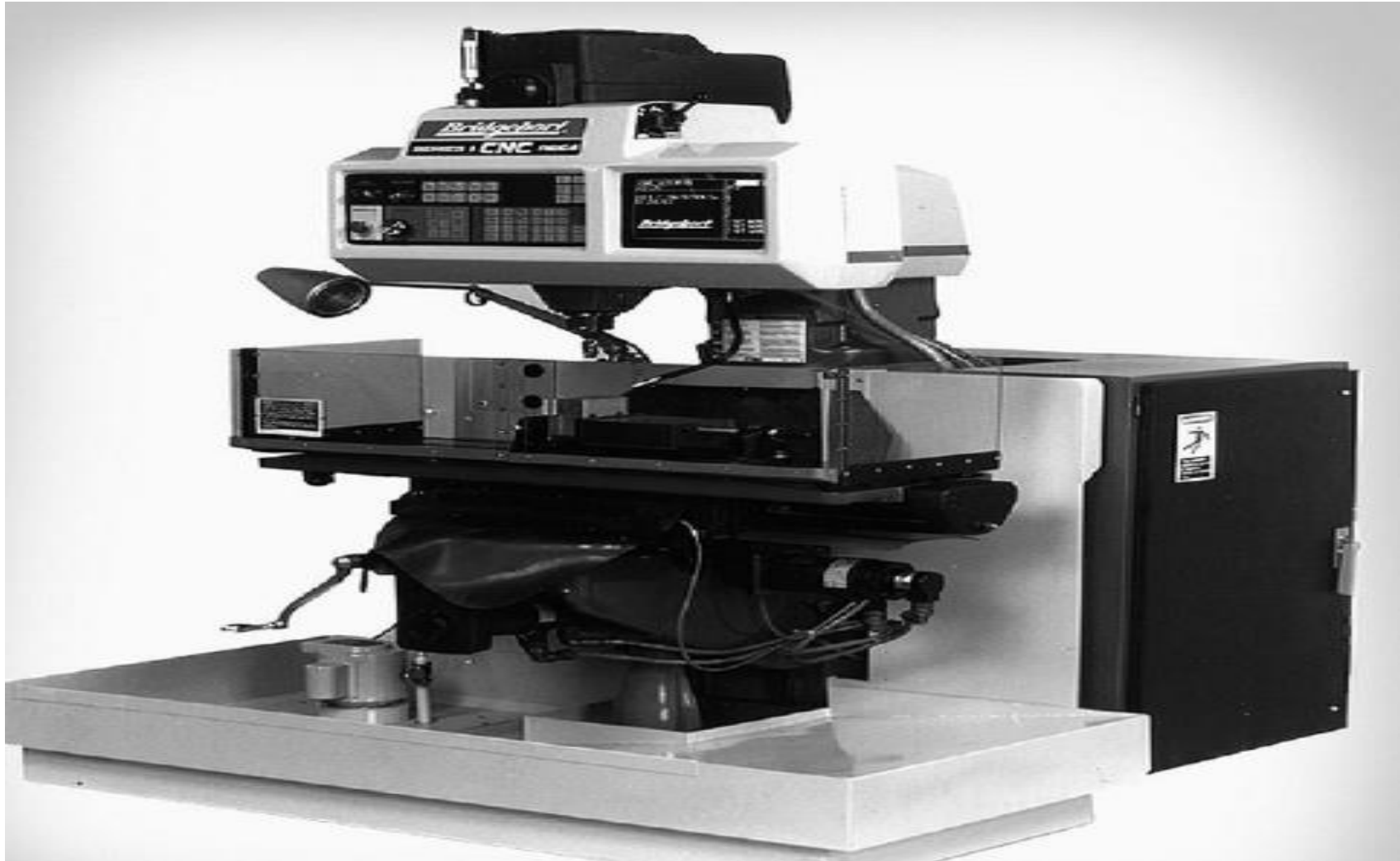
Figure 24.16 A computer numerical-control (CNC) vertical-spindle milling machine. This machine is one of the most versatile machine tools. The original vertical-spindle milling machine used in job shops is still referred to as a “Bridgeport”, after its manufacturer in Bridgeport, Connecticut. Source: Courtesy of Bridgeport Machines Division, Textron Inc.
