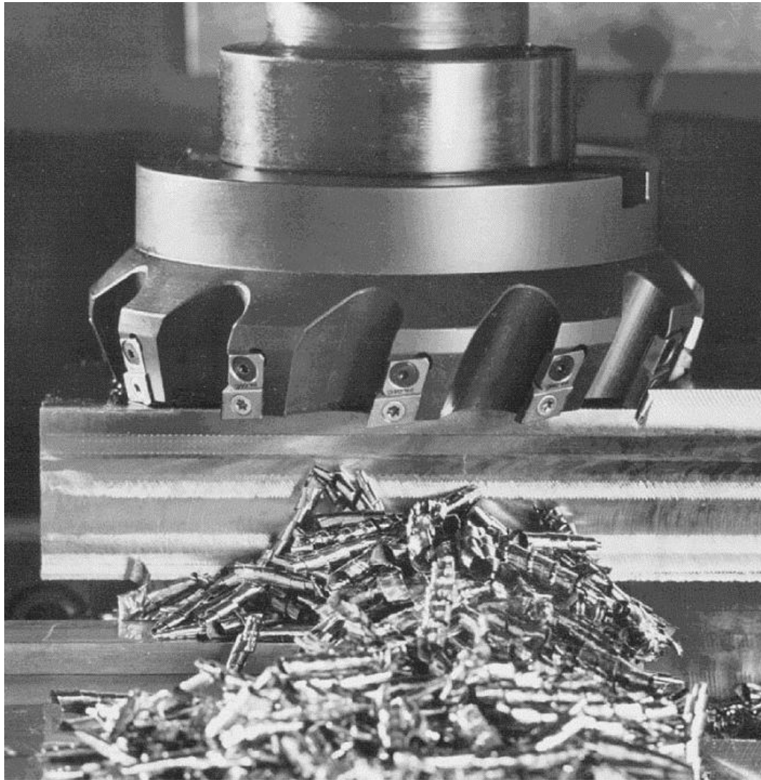
Figure 24.5 A face-milling cutter with indexable inserts. Source: Courtesy of Ingersoll Cutting Tool Company.
