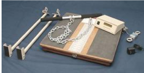
Figure 3.3: Jackson strength evaluation system
