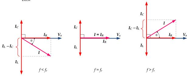
The bandwidth is again the interval between the half-power cut-off frequencies, which are the frequencies at which the current is  $\sqrt{2}$  of its minimum value. The cut-off frequencies for the parallel RLC circuit are given by:
