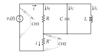
2. Set the function generator to produce a sinusoidal waveform (AC) with frequency of 6000 Hz, and *peak voltage* of  $V_p = 4$  V.
