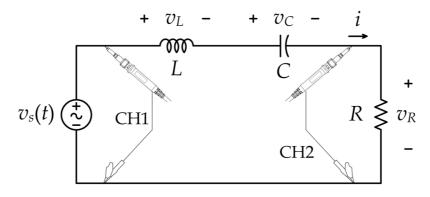
2. Set the function generator to produce a sinusoidal waveform (AC) with frequency of 6000 Hz, and *peak voltage* of  $V_p = 4$  V.
