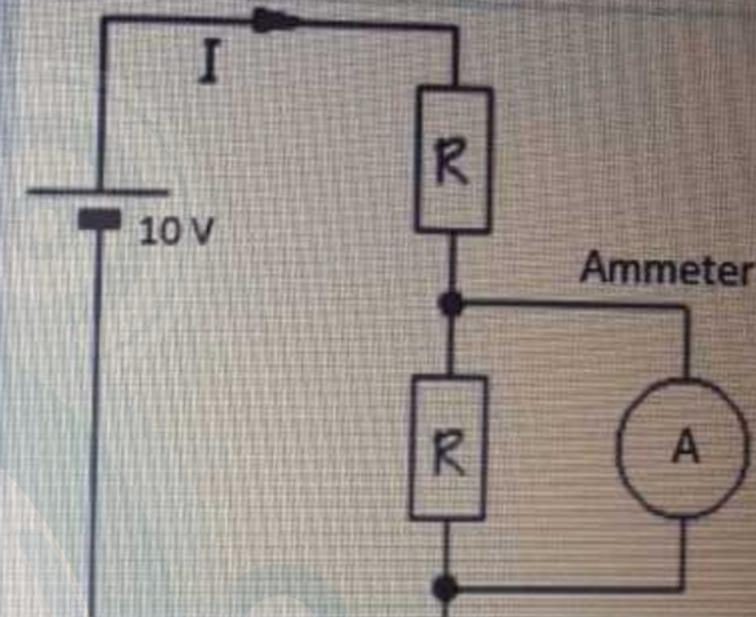
If  $R=180$  ohm, then the Ammeter reading (in Ampere) is:
