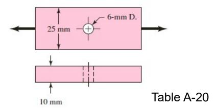
$$S_{ut} = 590 \text{ MPa}, S_y = 490 \text{ MPa},$$
