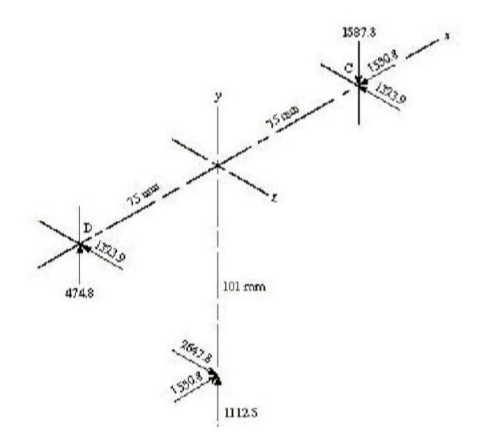
The radial load at D is The radial load at C is At D desired life is  $\sqrt{474.8^2 + 1323.9^2} = 1406.5N$   $\sqrt{1587.3^2 + 1323.9^2} = 2066.9N$
