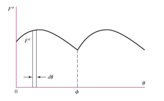
$$F_{\rm eq} = \left[\frac{1}{\phi} \int_0^{\phi} F^a d\theta\right]^{1/a} \qquad L_{\rm eq} = \frac{K}{F_{\rm eq}^a}$$
