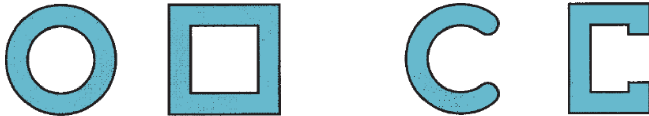
Figure 19.22 (a) Direct extrusion to produce a hollow or semi-hollow cross section; (b) hollow and (c) semi-hollow cross sections.
