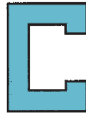
Figure 19.22 (a) Direct extrusion to produce a hollow or semi-hollow cross section; (b) hollow and (c) semi-hollow cross sections.
