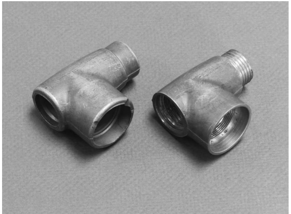
FIGURE 39.3 This plumbing fixture illustrates the basic and secondary processes. Casting (basic process) provides the starting geometry on the left, followed by a series of machining operations (secondary process) that accurately shape the holes and threads for the finished part on the right. (Courtesy of George E. Kane Manufacturing Technology Laboratory, Lehigh University.)
