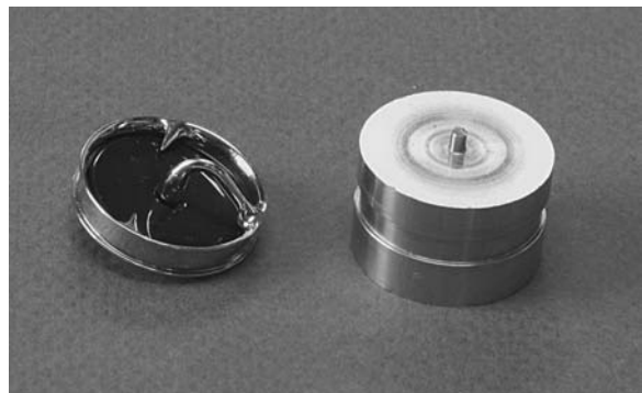
FIGURE 1.2 A mechanical heart valve on the left and the titanium workpiece from which the frame is machined on the right. (Courtesy of George E. Kane Manufacturing Technology Laboratory, Lehigh University.)
