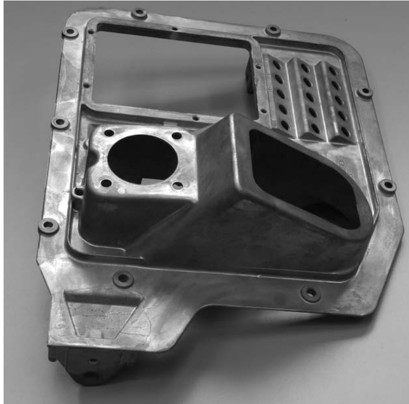
FIGURE 11.16 A large die casting measuring about 400 mm diagonally for a truck cab floor. (Courtesy of George E. Kane Manufacturing Technology Laboratory, Lehigh University.)
