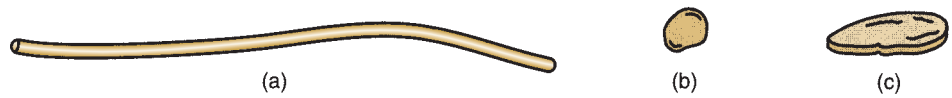
FIGURE 9.1 Possible physical shapes of imbedded phases in composite materials: (a) fiber, (b) particle, and (c) flake.
