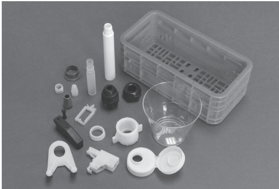
FIGURE 13.20 A collection of plastic injection-molded parts. (Courtesy of George E. Kane Manufacturing Technology Laboratory, Lehigh University.)
