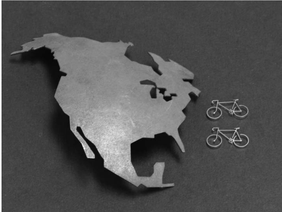
FIGURE 25.14 Parts produced by laser beam machining. The model bicycles on the right are about 20 mm (0.8 in) long. (Courtesy of George E. Kane Manufacturing Technology Laboratory, Lehigh University.)
