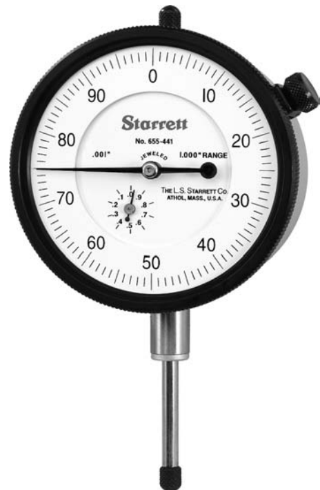
FIGURE 5.6 Dial indicator showing dial and graduated face. (Courtesy of L. S. Starrett Co.)
