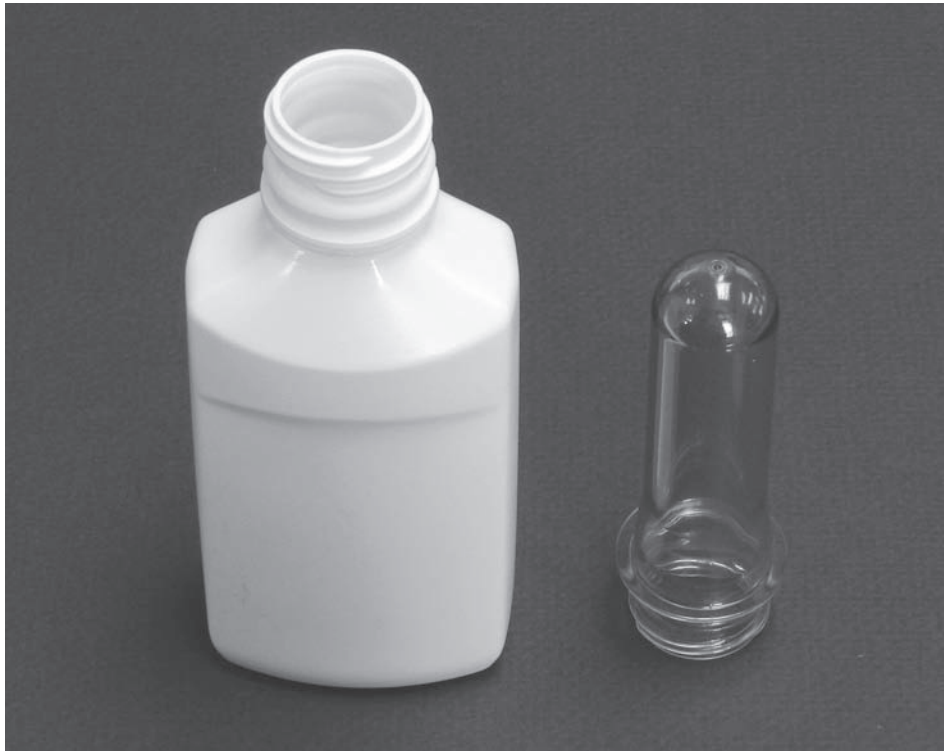
FIGURE 13.34 An injection blow molded bottle on the left and a parison for a similar part on the right. (Courtesy of George E. Kane Manufacturing Technology Laboratory, Lehigh University.)
