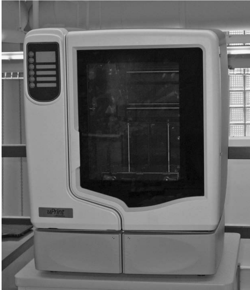
FIGURE 32.8 Fused deposition modeling machine. (Courtesy of George E. Kane Manufacturing Technology Laboratory, Lehigh University.)
