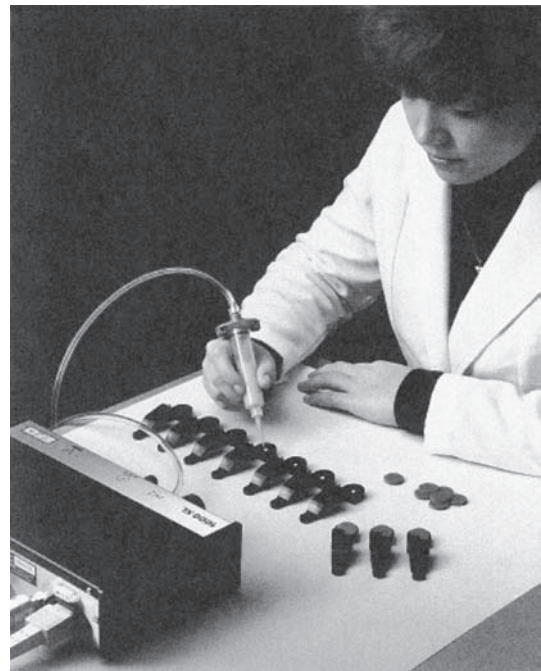
FIGURE 30.13 Adhesive is dispensed by a manually controlled dispenser to bond parts during assembly. (Courtesy of Nordson, Inc.)
