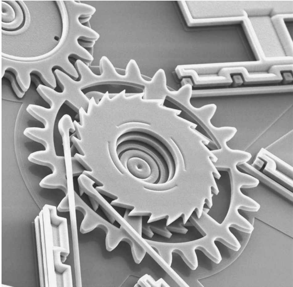
FIGURE 35.2 Microscopic ratchet mechanism fabricated of silicon (Photo courtesy of Paul McWhorter).
