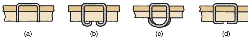
FIGURE 31.15 Common types of wire stitches: (a) unclinched, (b) standard loop, (c) bypass loop, and (d) flat clinch.
