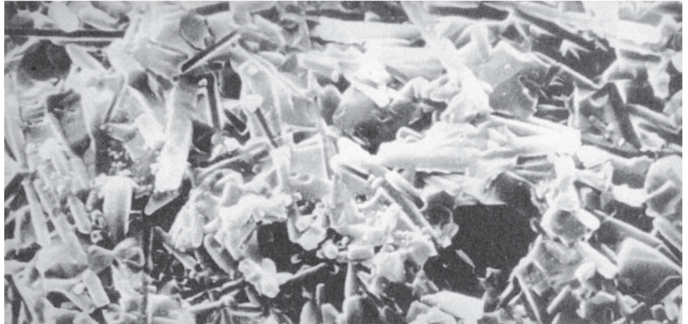
FIGURE 9.10 Highly magnified electron microscopy photograph (about 3000X) showing fracture surface of SiC whisker reinforced ceramic ( \text{Al}_2\text{O}_3 ) used as cutting tool material. (Courtesy of Greenleaf Corporation.)
