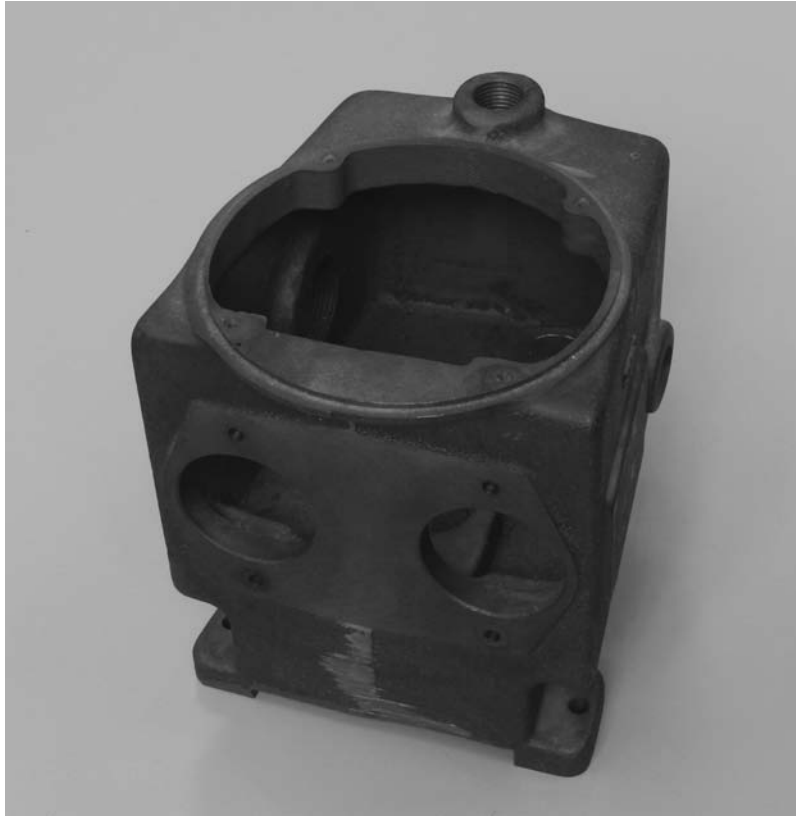
FIGURE 11.1 A sand casting for an industrial pump. Holes and surfaces have been machined. (Courtesy of George E. Kane Manufacturing Technology Laboratory, Lehigh University.)
