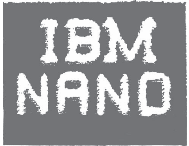
FIGURE 36.3 An atomic force microscope image of silicon dioxide letters on a silicon substrate. The oxide lines of the letters are about 20 nm wide. (Image courtesy of IBM Corporation.)
