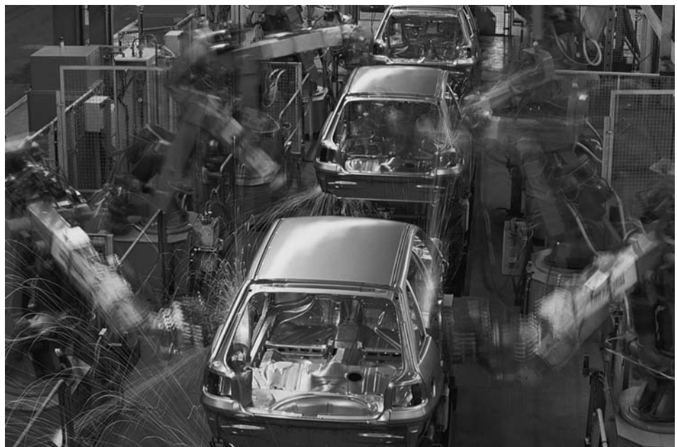
FIGURE 37.16 A portion of an automobile assembly line in which robots perform spot-welding operations. (Photo courtesy of Ocean/Corbis Images.)
