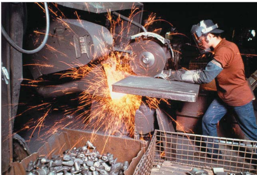
Metal saws, such as this one, require time to changeover from one product to the next. The depth and length of the cut must be adjusted and the blade itself may have to be changed.
