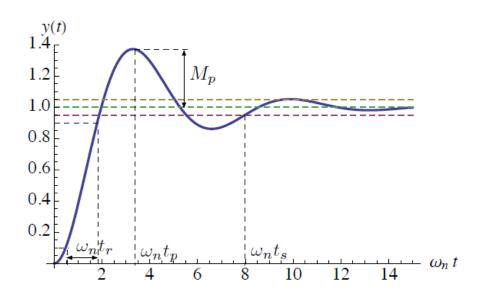
Rise time  $t_r$  — hard to calculate analytically. Empirically, on the normalized time scale  $(t \to \omega_n t)$ , rise times are approximately the same
