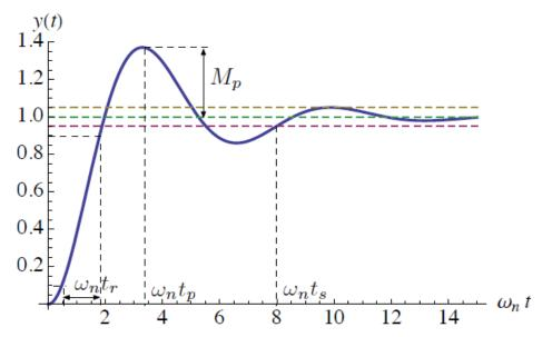
$$t_s = \min \left\{ t > 0 : \frac{|y(t') - y(\infty)|}{y(\infty)} \le 0.05 \text{ for all } t' \ge t \right\} \text{ (here, }$$
