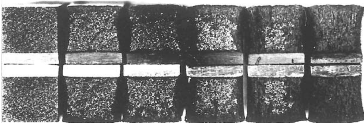
Figure 8.14 Photograph of fracture surfaces of A36 steel Charpy V-notch specimens tested at indicated temperatures (in ° C).
