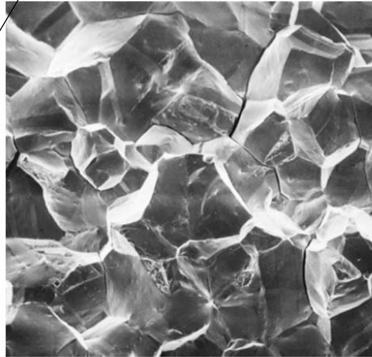
Figure 8.7 (a) Schematic cross-section profile showing crack propagation along grain boundaries for intergranular fracture. (b) Scanning electron fractograph showing an intergranular fracture surface.
