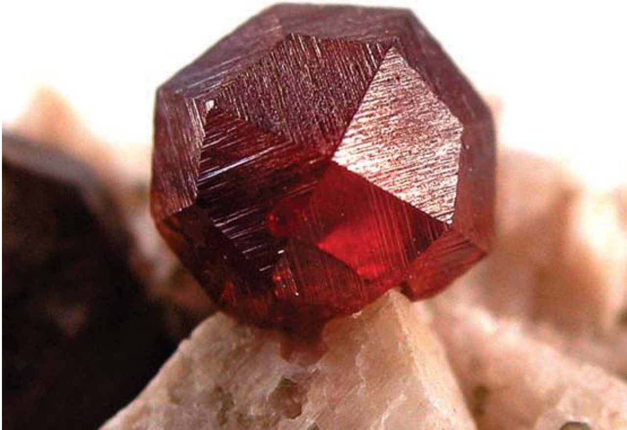
Figure 3.17 Photograph of a garnet single crystal that was found in Tongbei, Fujian Province, China.
